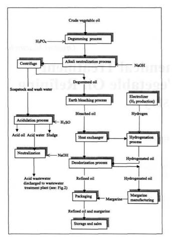
Fig. 1. Simplified schematic diagram of vegetable oil refining processes: sources of vegetable oil refinery wastewater (acid and technological wastewater).
