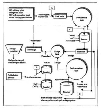
treatment system for the vegetable oil refinery wastewater. Sampling locations: A, technological wastewater; B, acid wastewater; C, intermediate wastewater; D, final treated wastewater.
