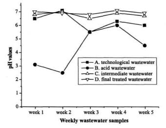
Fig. 3. Variations of wastewater pH values. Each of the results shown is represented by a mean value of 3 samples taken each week for 5 weeks.
